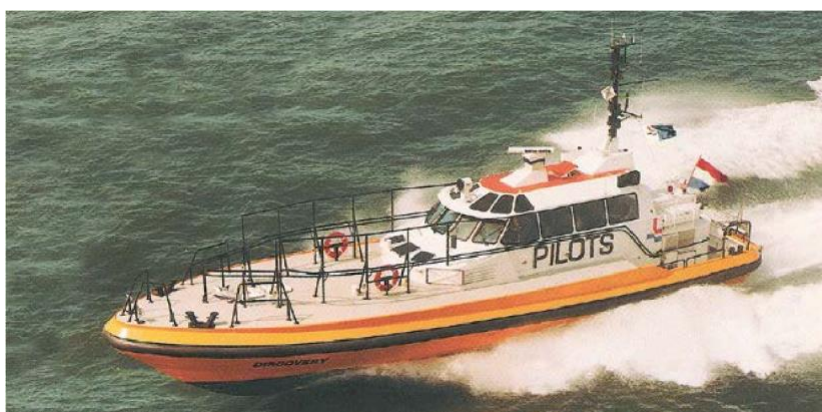
M The yacht Alcedo, based on a traditional fishing boat with leeboards, during her maiden voyage. Tightly built and finished and with great care. N Fast aluminium pilot tender. NN Harbour police cutter.
