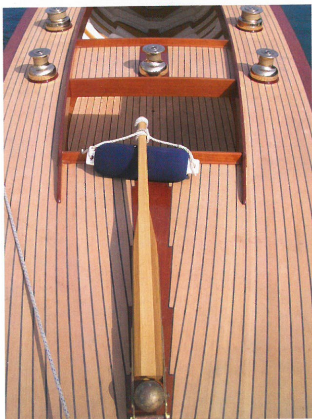
Above: Note the two strong ring frames in way of Valdai's mast Left: Redecked, and sporting new Meissner winches
